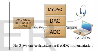
The 3 stations were set to frequencies of 16 kHz, 26 kHz and 51.1 kHz while the message signal had a frequency of 3 kHz. Additive White Gaussian Noise (AWGN) was also injected into generated AM signal.
