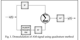
method was employed based on (1). The LabView code for the demodulation is represented in *Fig. 3*. The received AM signal is squared and added to the Hilbert transformed version of the same signal. The square root of the resultant waveform is used to derive the original message.
